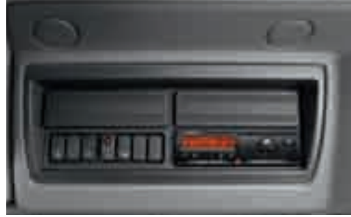
The tachograph is practically positioned in the header shelf.
