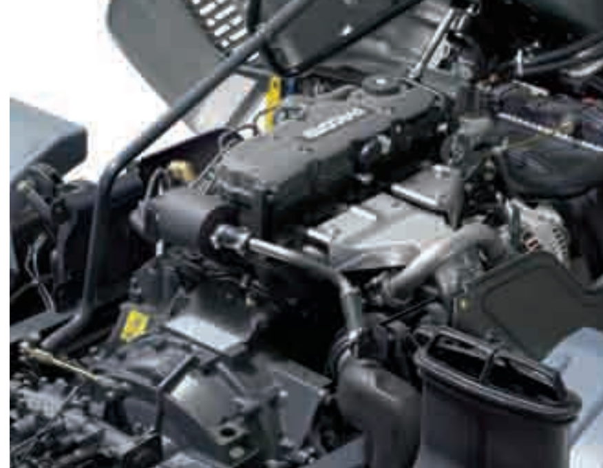
The 4.5 litre four cylinder PACCAR FR engine is available with outputs from 140 hp to 185 hp.
